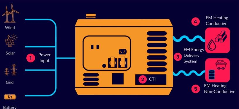
By coupling electromagnetic (EM) energy directly to materials being heated, EMPowered Heat requires 40% - 60% less energy to operate and is economic at industrial scale, high temperature, or high power.
